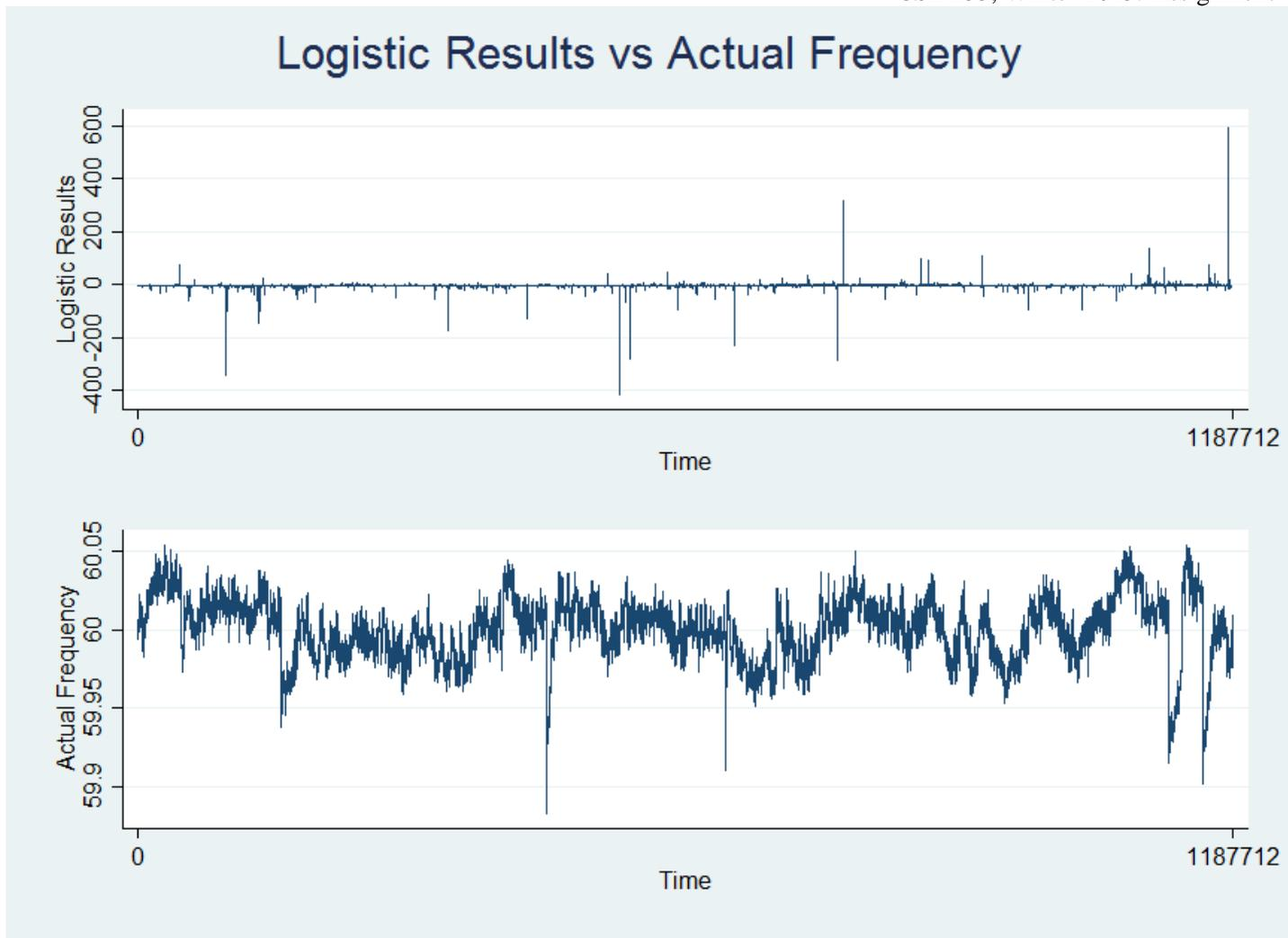
FIGURE 10: Logistic Regression Results versus actual Frequency. Higher logistic results supposedly indicate an oncoming frequency instability event. Testing sample compose of 12 different samples throughout October 2014.
